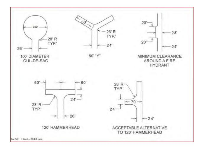
**(114)** "D103.4 Dead ends. Amend to read: Dead-end fire apparatus access roads shall be provided with width and turnaround provisions in accordance with Table D103.4 and 503.2.5.
