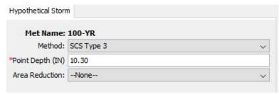
Figure 4: 100-yr Storm Meteorologic Model Inputs
